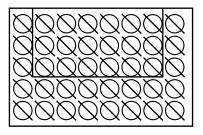
Turbulator Positions in Heat Exchanger 235 & 275 Cabinets. 40 off
